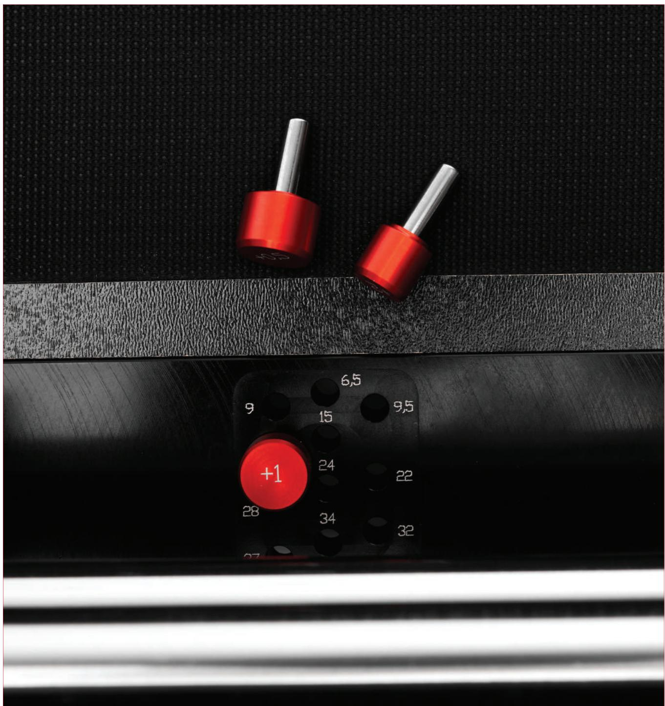
Underneath the metric scales, there are bases with holes for positioning pins. Their purpose is to facilitate the positioning of furniture boards for drilling in the plane. The set includes neutral pins as well as +0.5/1.5/2 mm pins, which increase the distance between the workpiece and the hole accordingly.
