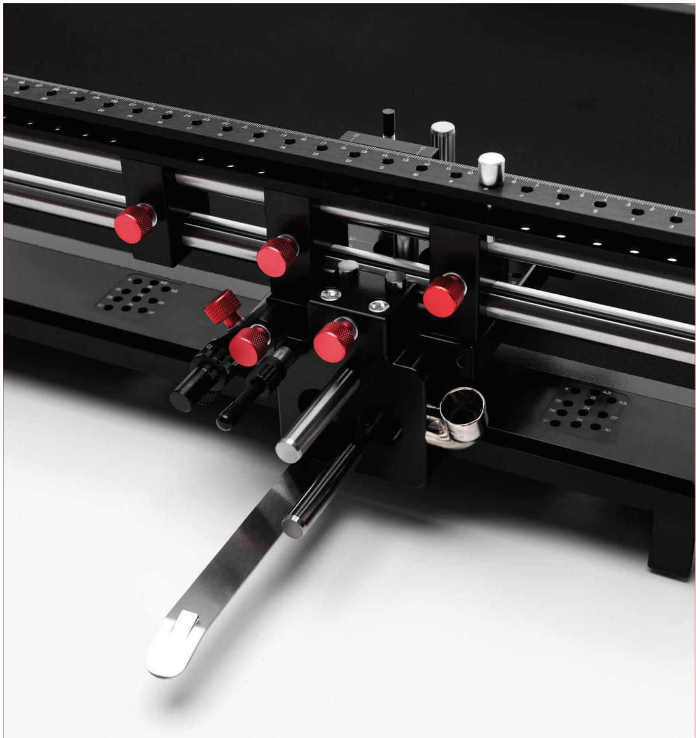
The table is equipped with inserts for **drilling in the edges**, which are mounted at the rear of the movable positioners.
