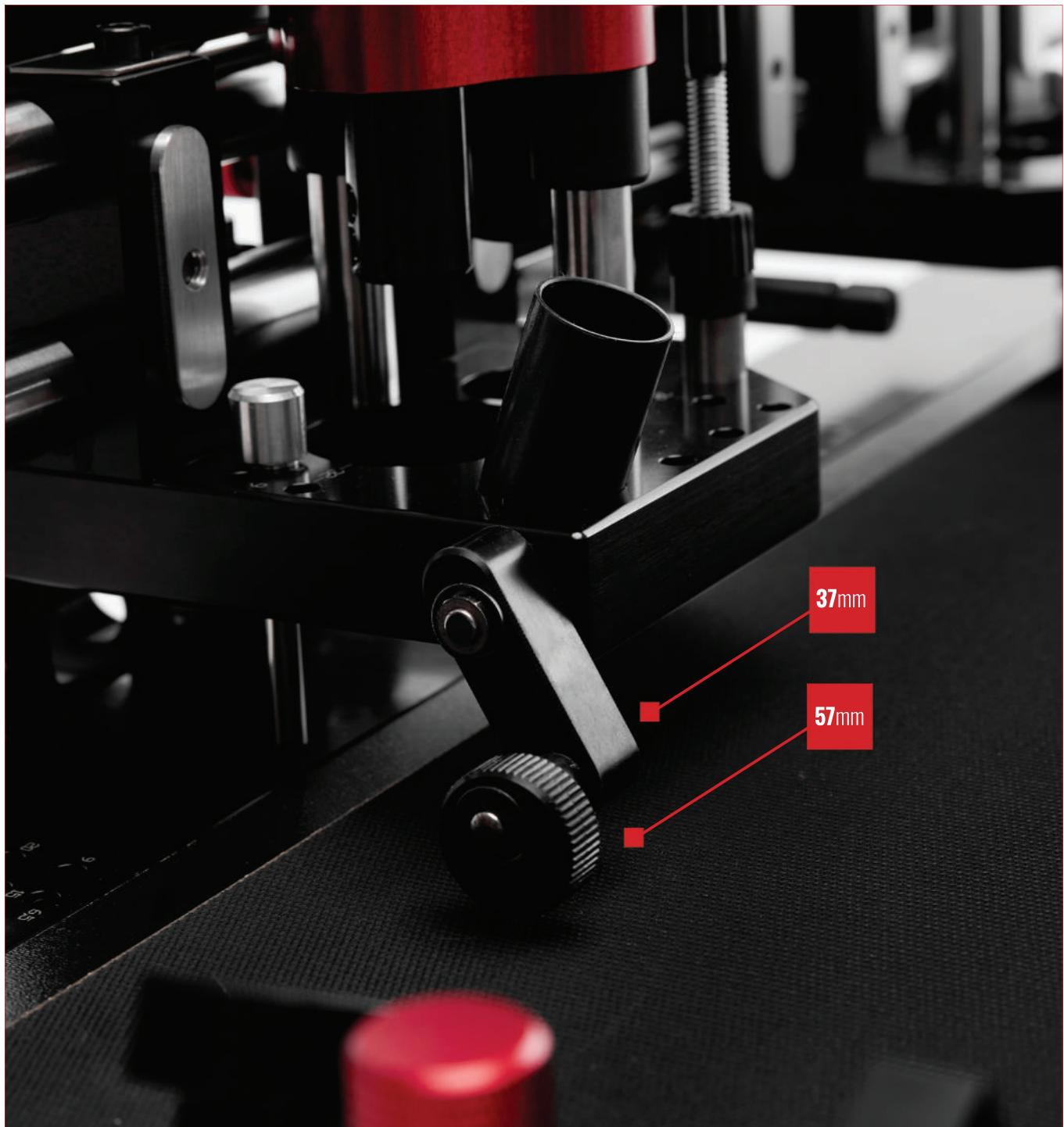
Next to the positioning sliders that move along the metric scales, there are additional positioning bases for drilling elements at distances of **37** and **57 mm** from the drill axis.
